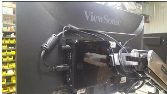
4. Run CAT6 cable from hub to NUC and connect both ends.
